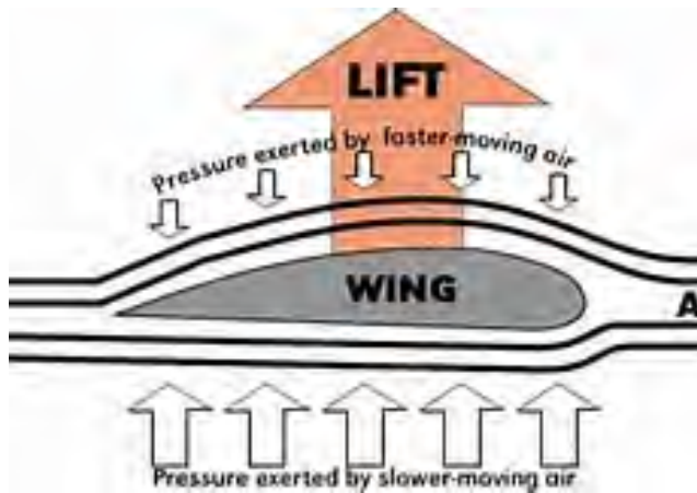
Bernoulli Effect on an AerFoil or Aircraft Wing Lift & Weight combined with Thrust & Drag (The 'A' is 'Direction Of Air Flow')
